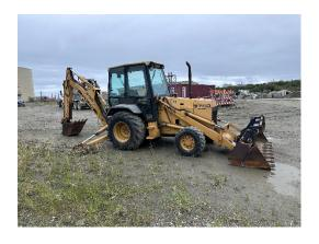
**1995 Ford 575DF1 Backhoe** known issues include: Electrical, pistons and rings, valve seals Windows, worn out pins and bushings on Digger arm. Will not run at the moment.
