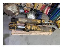
CAT Hydraulic Lift Cylinder Assembly (3G5495 & 3G5496) fits CAT loaders 966D, 966E, 966F and 966FII. Needs to be resealed.
