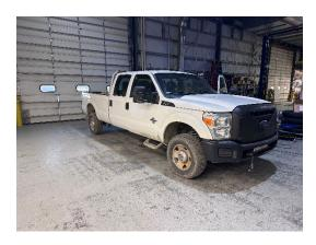
Ford F350 Crew Cab known issues include: Front axle bearings and seals, front drive line maintained, Leaking valve cover gasket on engine, Oil leak under turbo, front and rear suspension. Currently runs.
