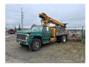
1977 Ford F-750 Pole Truck known issues include: Transmission, little to no brakes, exhaust leak, hydraulic leak on the pole claw, Holes in floor, gas tank rusted. 50 years old. Known to start and run.
